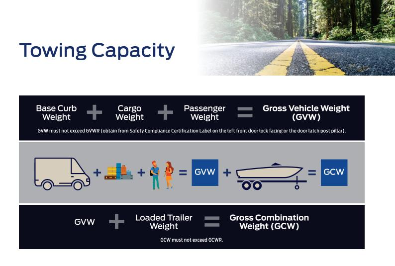
Gross Combination Weight (GCW) is the weight of the loaded vehicle (GVW) plus the weight of the fully loaded trailer. It is the actual weight obtained when the vehicle and trailer are weighed together on a scale.
